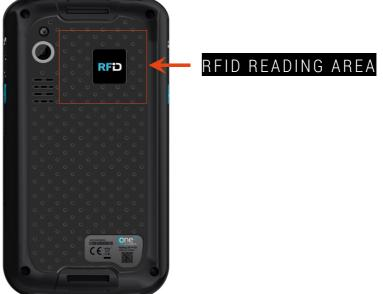
C-One<sup>2</sup> LF AGRIDENT with RFID options to read, please put the TAG/CARD on the RFID area.
